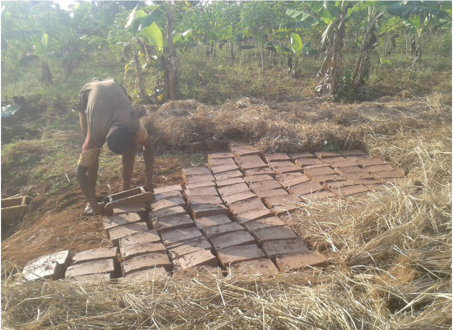
5. The traditional way of making clay bricks in Uganda, using a jig and letting them dry in the sun / Author's own 2016
