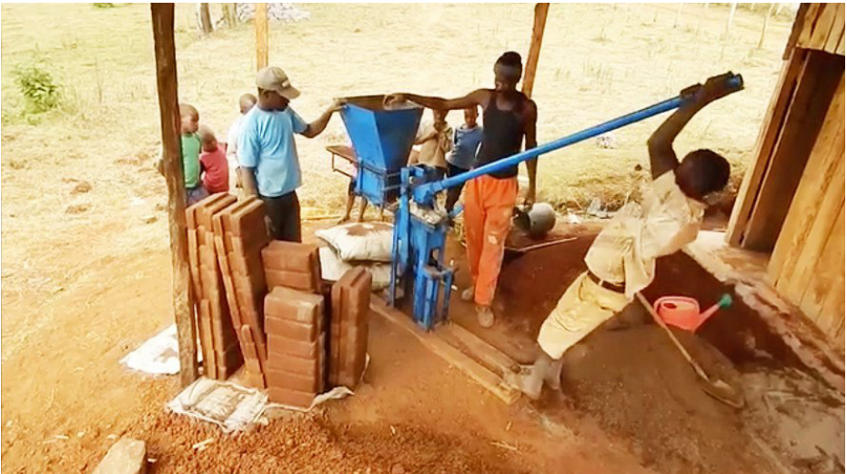
6. A hand powered compressed earth brick press that produces stronger, more precise earth bricks / DiSatsio 2015
